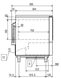
Drain Electrical inlet (power)
